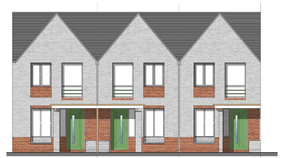
Front Elevation showing Materials
